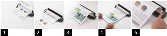
**1** Insert the page face up and press the Scan button. **2** The iX100 proceeds to scan the front side. **3** The page exits facing front side down. **4** Reinsert the page without pressing the Scan button. **5** The page is scanned. Press the Scan button to end the scanning process and create the PDF image file.
